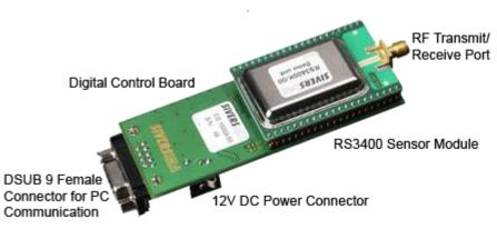
Figure 2. Controller board and radar sensor
